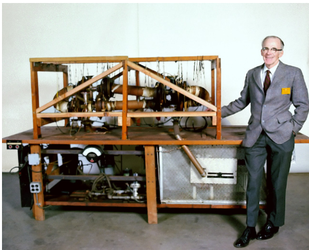
Figure 13. Lyman Spitzer with the Model A stellarator that was exhibited at Geneva 1958. Courtesy of the Princeton Plasma Physics Laboratory.
