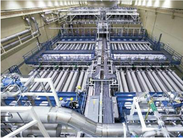
Figure 19. One of two NIF laser bays. System has been test fired at 1.1 MJ per pulse. Courtesy of Lawrence Livermore National Laboratory (LLNL).
